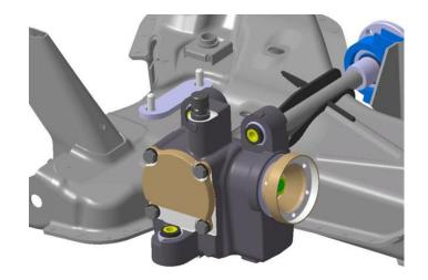
A mechanical assembly transmitting the engine torque to the longitudinal transmission by means of a bevel gear.
