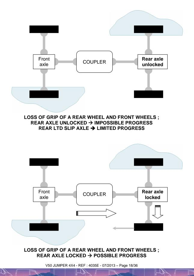
In free position, the Dangel rear axle distributes the torque symmetrically between the right wheel and the left wheel. Moreover, the differential allows the right rear wheel and the left rear wheel to turn at different speeds. In bends, this guarantees a robust drive performance, and preserves the transmission and tyres.
