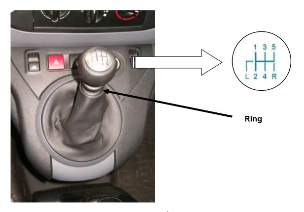
The lower speed (L) is located next to the  $2^{nd}$  gear. In order to engage it, unlock the safety by lifting the ring. It can only be used in 4-wheel drive mode.
