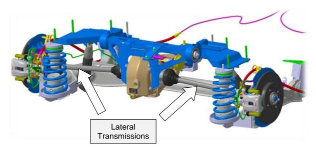
They transmit the engine torque from the differential to the wheels.
