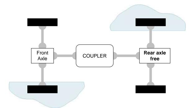
LOSS OF GRIP OF A REAR WHEEL AND OF A FRONT WHEEL; REAR AXLE FREE → FORWARD MOVEMENT IS IMPOSSIBLE
