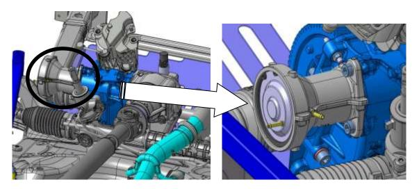
Mechanical assembly allowing switching between 2WD and 4WD using the nob on the dashboard.
