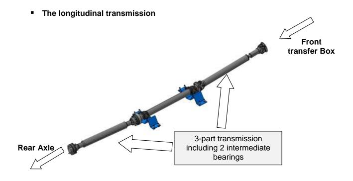
Mechanical element that transmits the engine torque to the rear wheels through a visco-coupler.
