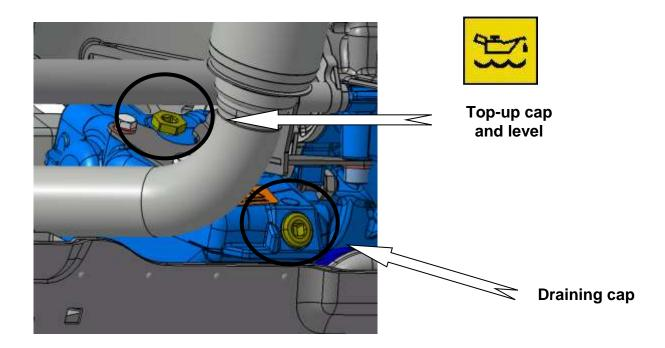
Note: The filling can also be done through the breather, in this case, open the filler cap to control the level.
