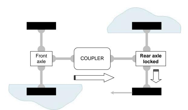
LOSS OF GRIP OF A REAR WHEEL AND OF A FRONT WHEEL; REAR AXLE LOCKED → FORWARD MOVEMENT IS POSSIBLE
