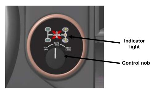
For your safety, the system prevents locking the differential at speeds over approximately 30 km/h.
