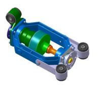
Permanently active, it detects the loss of grip of the front wheels and then transmits the engine torque to the rear wheels.
