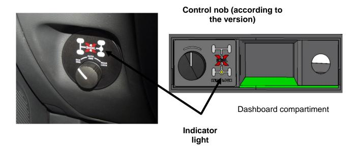
For your safety, the system prevents locking the differential at speeds over approximately 30 km/h.
