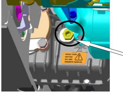
The filling plug indicate the oil level
