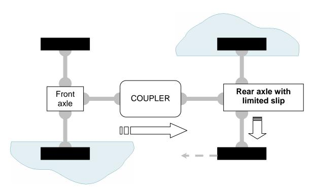
LOSS OF GRIP OF A REAR WHEEL AND OF A FRONT WHEEL; REAR LTD SLIP AXLE → FORWARD MOVEMENT IS POSSIBLE Limited to 80 N.m of torque at the wheel.
