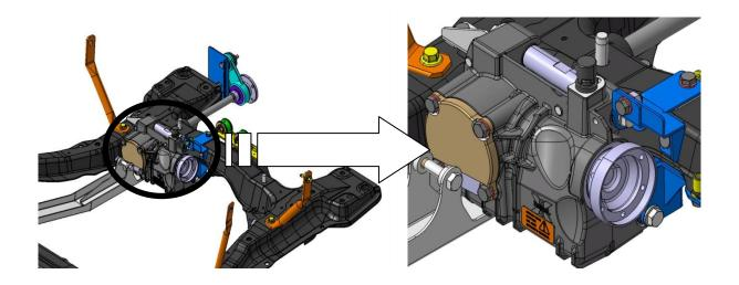
A mechanical assembly transmitting the engine torque to the longitudinal transmission by means of a bevel gear.
