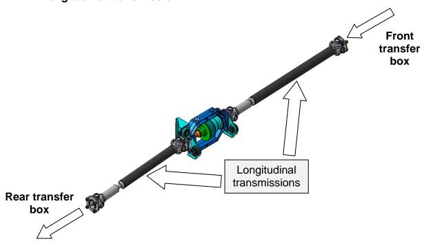
A mechanical assembly transmitting the engine torque to the rear wheels by means of a coupler.
