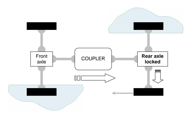
LOSS OF GRIP OF A REAR WHEEL AND FRONT WHEELS;
