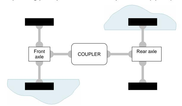
LOSS OF GRIP OF A REAR WHEEL AND OF A FRONT WHEEL; FREE REAR AXLE → FORWARD MOVEMENT IS IMPOSSIBLE
