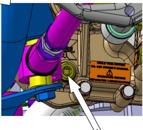
The filling plug does not indicate the oil level
