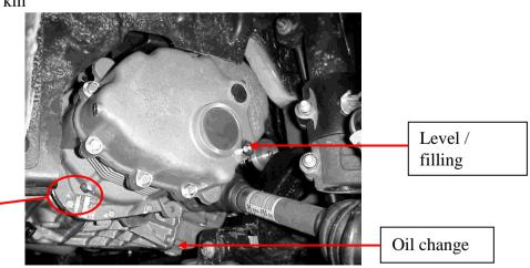
Nota: when replacing a transfer bo or a rear axle by a new part, the 1<sup>st</sup> oil change between 1500 and 2500 km is compulsory.
