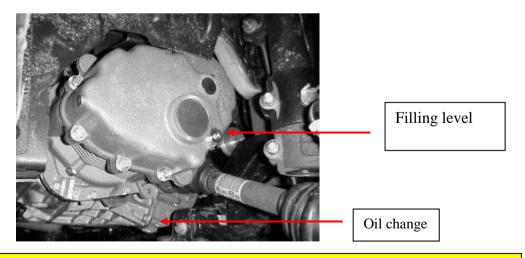
Note: when replacing a transfer box or rear axle by a new part, the 1<sup>st</sup> oil change between 1,500 and 2,500 km is compulsory.
