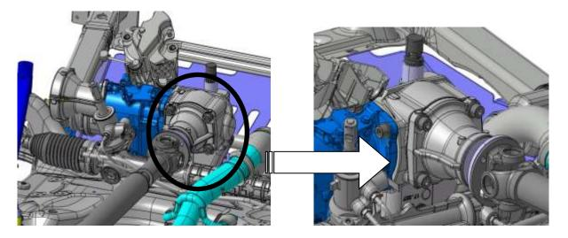
Mechanical assembly that transmits the engine torque to the longitudinal transmission through an angle transmission.
