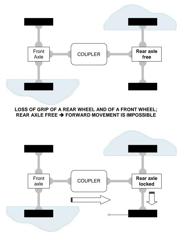
LOSS OF GRIP OF A REAR WHEEL AND OF A FRONT WHEEL; REAR AXLE LOCKED → FORWARD MOVEMENT IS POSSIBLE
