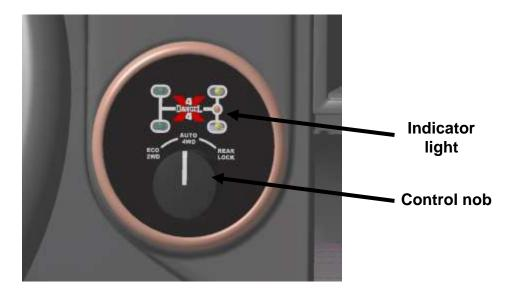
For your safety, the system prevents locking the differential at speeds over approximately 30 km/h.
