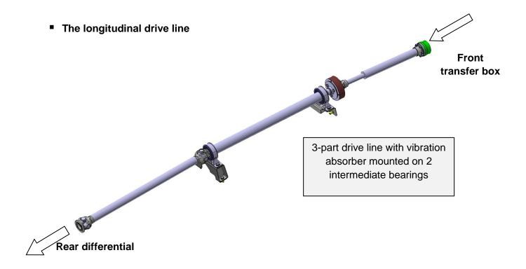
Mechanical assembly that transfers the engine torque to the rear wheels through a visco-coupler.
