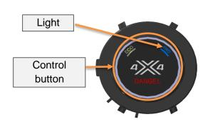
While driving switching from ECO position to 4WD / AUTO 4WD position is possible, **EXCEPT if the front wheels are slipping**.
