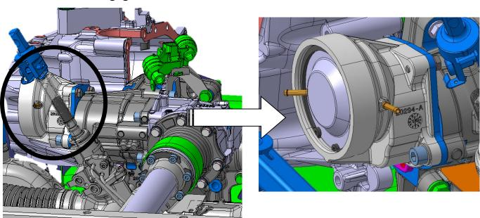
Mechanical assembly allowing switching from 2WD to 4WD using the knob on the dashboard.
