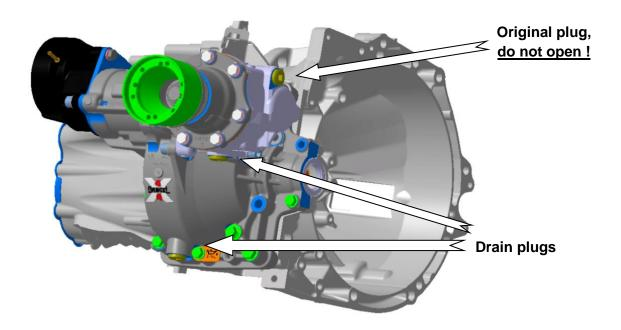
Note: it is imperative to open both drain plugs to empty completely the remaining oil of the transfer box.
