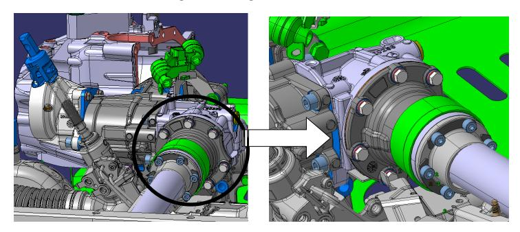
Mechanical assembly that transfers the engine torque to the longitudinal drive line through a transfer box.
