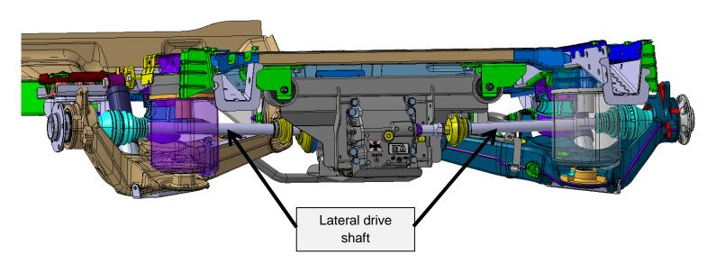
They transfer the engine torque from the differential to the wheels.
