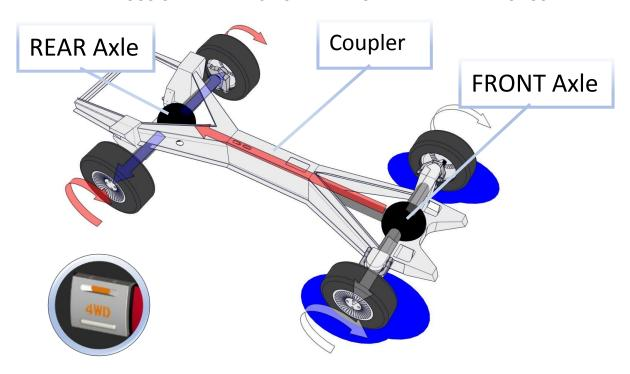
Functioning of Rear LOCK (option rear differential WITH locking)
