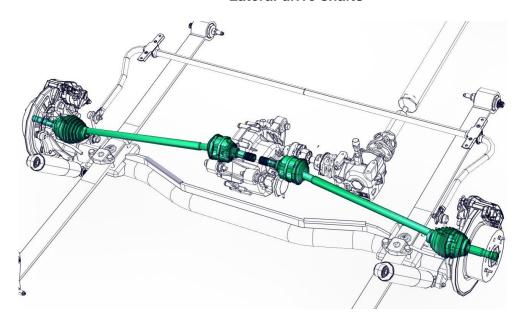
They transfer the engine torque from the differential to the wheels.
