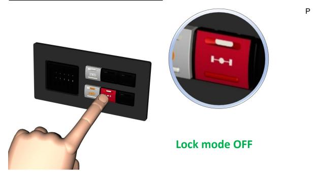
press the control switch again to unlock the rear differential. Audible and light signals
