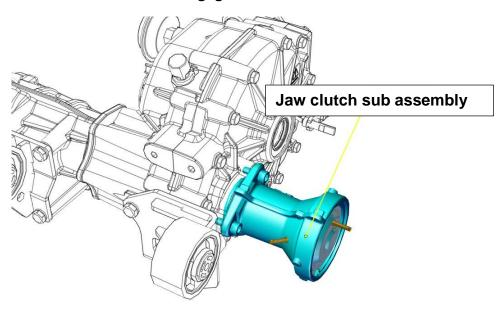
Mechanical assembly allowing switching from 2WD to 4WD using the switches on the dashboard.
