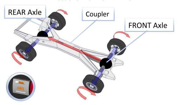
The operation of the 4 wheel drive system designed and constructed by Automobiles DANGEL is based on **automatic and optimum distribution** of the **engine torque** with the **coupler** at the **heart of the system**.
