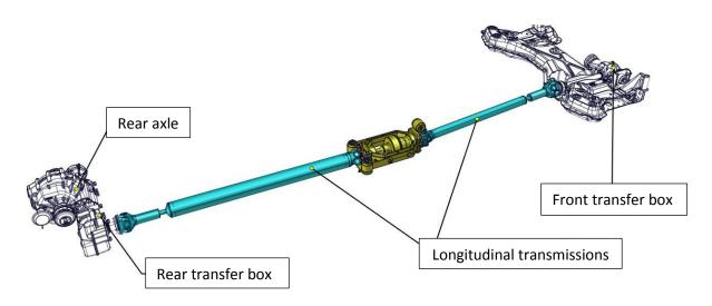
Mechanical assembly transmitting the engine torque to the rear wheels by means of a coupler.
