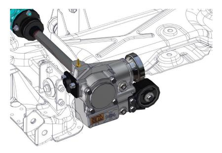
Mechanical assembly transmitting the engine torque to the longitudinal transmission by means of a bevel gear.
