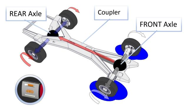
Functioning of Rear LOCK (option rear differential WITH locking)
