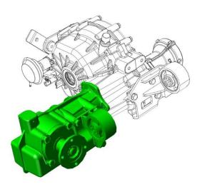
Mechanical assembly transmitting the engine torque to the rear axle by means of a bevel gear.
