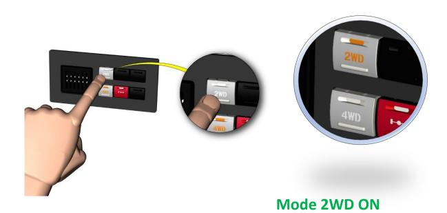
Press the 2WD switch, the orange indicator light above it comes on when 2WD is activated.
