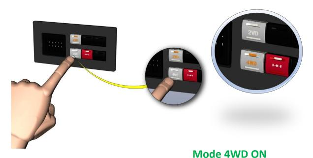
Press the 4WD switch, the orange indicator light above it comes on when 4WD is activated.
