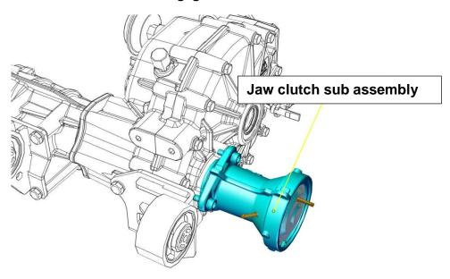
Mechanical assembly allowing switching from 2WD to 4WD using the switches on the dashboard.
