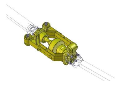
Permanently active, it detects the loss of grip of the front wheels and then transmits the engine torque to the rear wheels. The coupler will adjust the percentage of torque as required.
